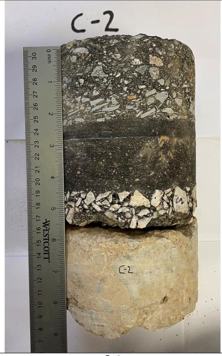
C-2 Asphalt Thickness (5½") Concrete Thickness (3") Stone Base (6½")
